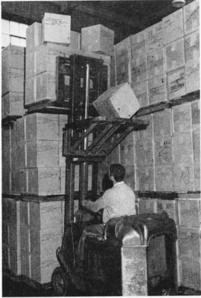
This scene arranged to simulate a condition typical in storage areas where high stacking is the regular order because storage space is at premium shows how the new type of guard installed on the fork-lift jitney in Case IV "stopped" the falling box from "conking" the jitney driver.
